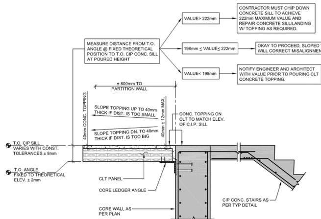
Figure 14: Detail at Core Sill
