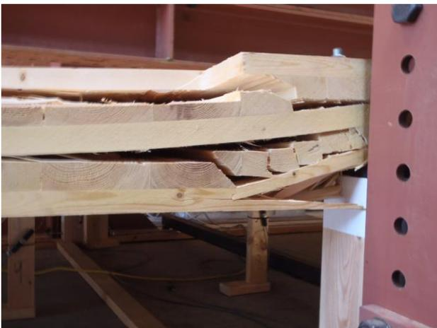
**Figure 9:** CLT Shear Failure at Support
