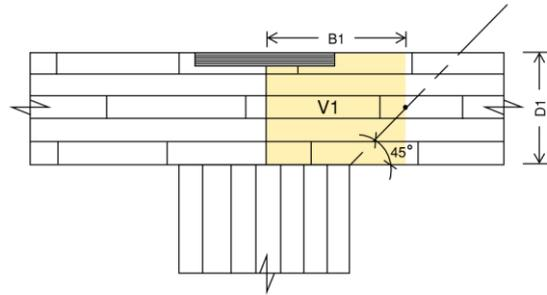
Figure 6: V1 or V3 Shear Area
