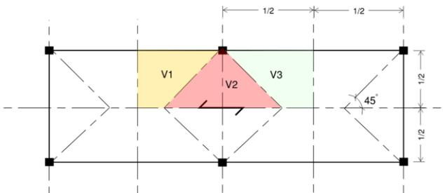
Figure 5: Plan View of CLT Panel – Shear Approximation
