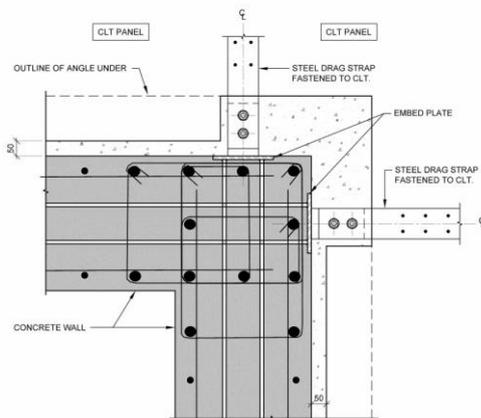
Figure 11: Drag Strap Detail at Core
