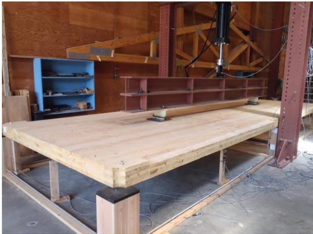
**Figure 8:** CLT Testing Apparatus
