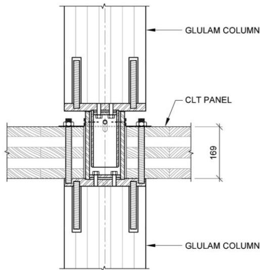
Figure 13: Column to Column Connection
