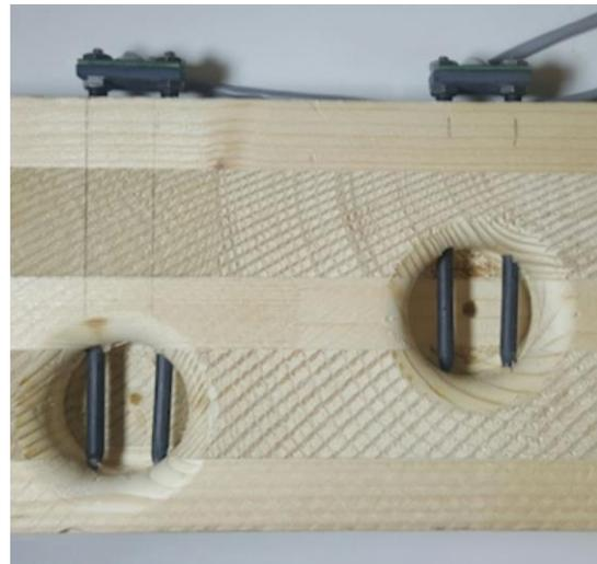
Figure 18: Moisture Meter Probes
