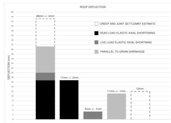
Figure 12: Cumulative Axial Shortening at Roof
