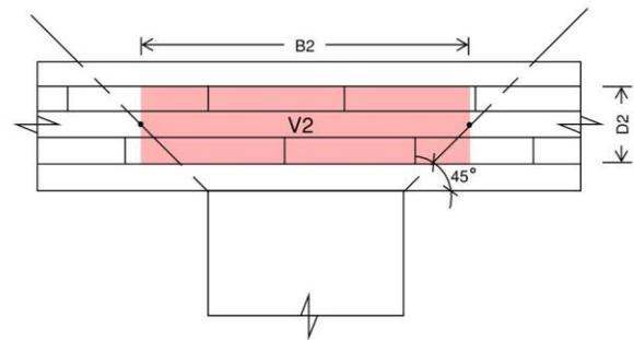
Figure 7: V2 Shear Area
