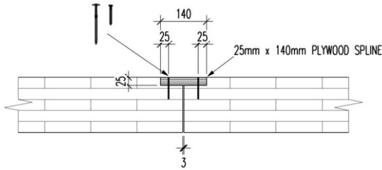
Figure 10: CLT Spline Detail
