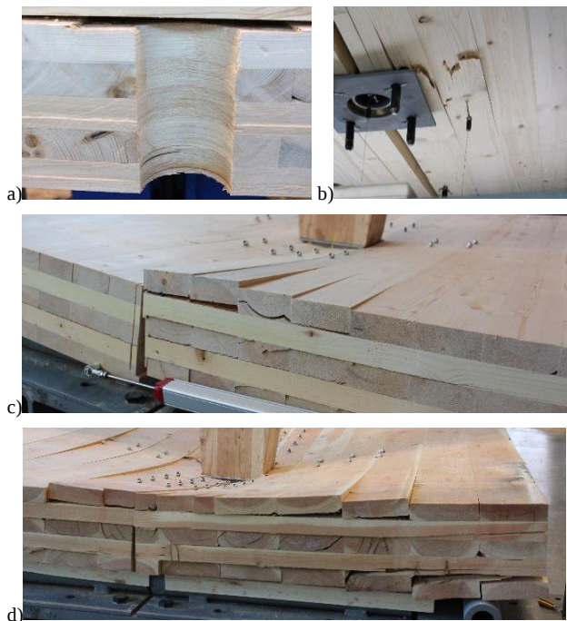
Figure 4. The vicinity of the point-support after unloading (a); tensile failure of the underside boards (b); failure at interface of single layers outside the reinforced zones in S21 (c); and failure outside the point support zone of the repaired panels (d).
