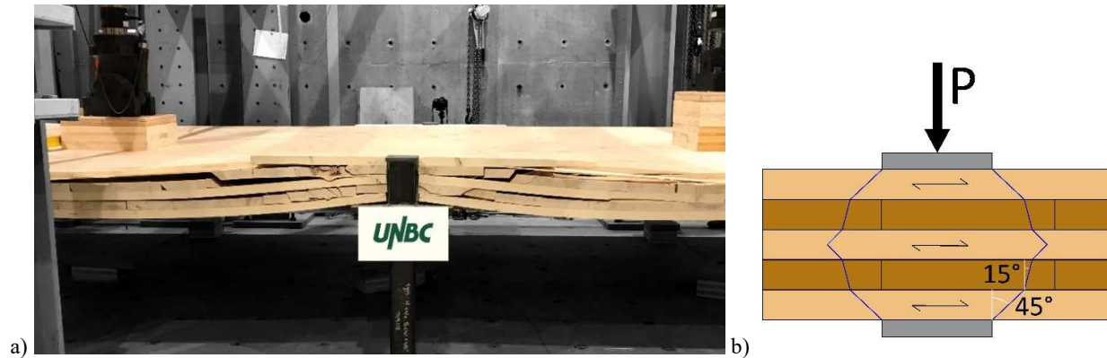
Figure 1. Point-supported CLT punching shear failure (a); CLT load dispersion model (b).
