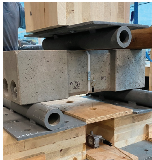
Figure 6 – Structural Testing with Steel Roller Supports
