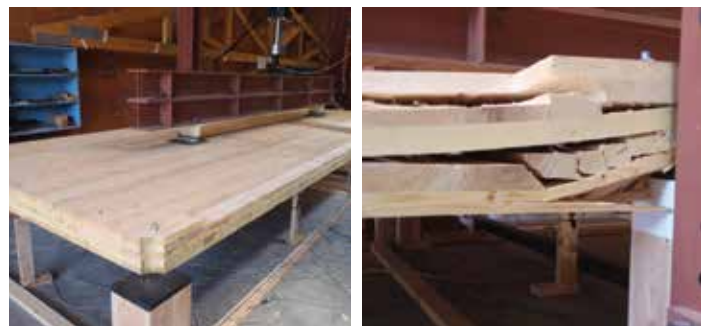
Figure 3. Point supported CLT panel testing apparatus (left); Failure (right).
