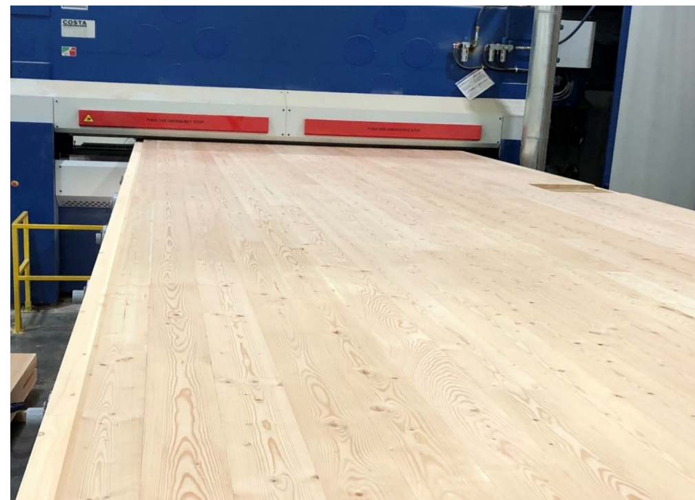
Photo of 7-ply CLT in Production. (Kalesnikoff)
