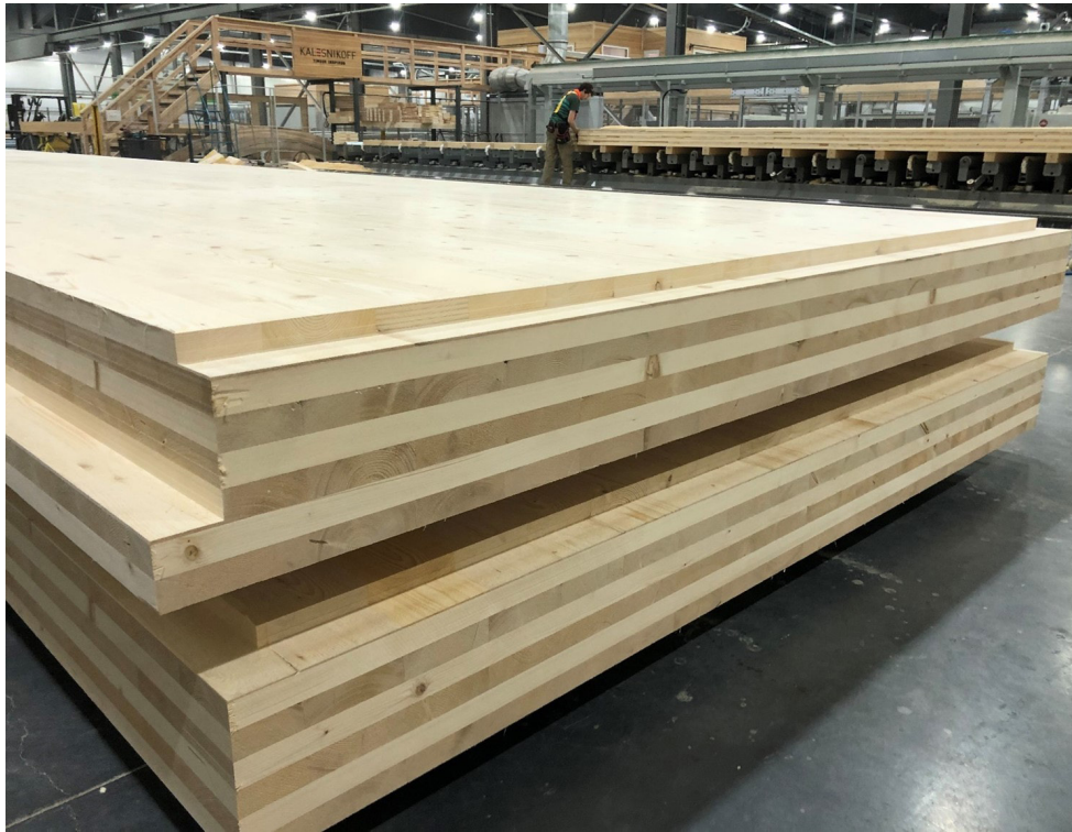
Photo of 7-ply CLT in Production. (Kalesnikoff)
