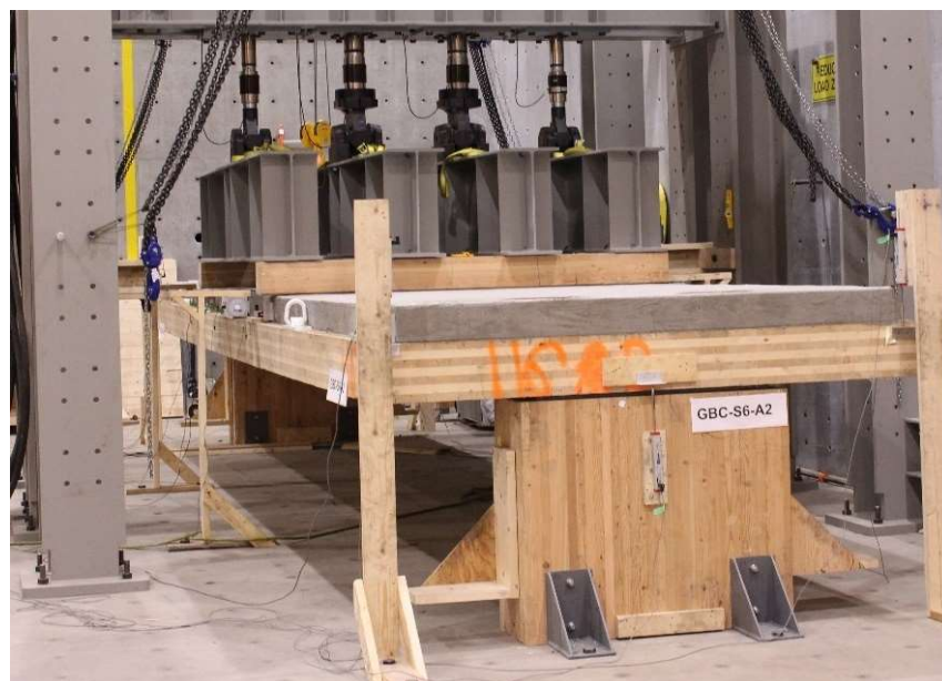
Figure 4. Test Setup of a Full-Scale TCC Floor
