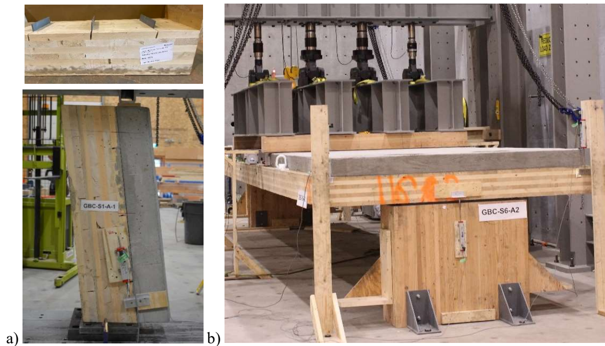
Figure 6. (a) Connector tests; (b) Full-Scale TCC Floor
