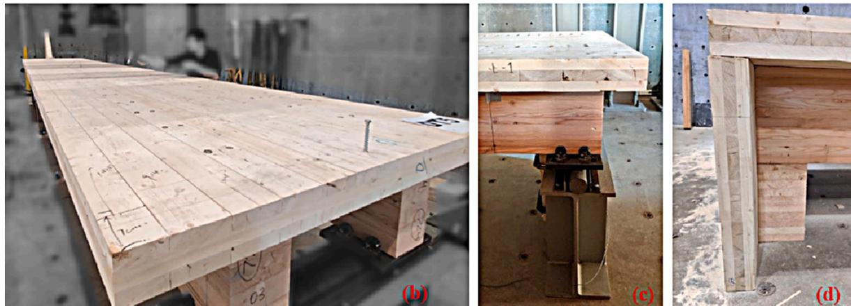
Fig. 7. (a) Impact hammer modal test and analysis, (b) T-beam specimen under test; (c) roller end supports, (d) wall/beam support.
