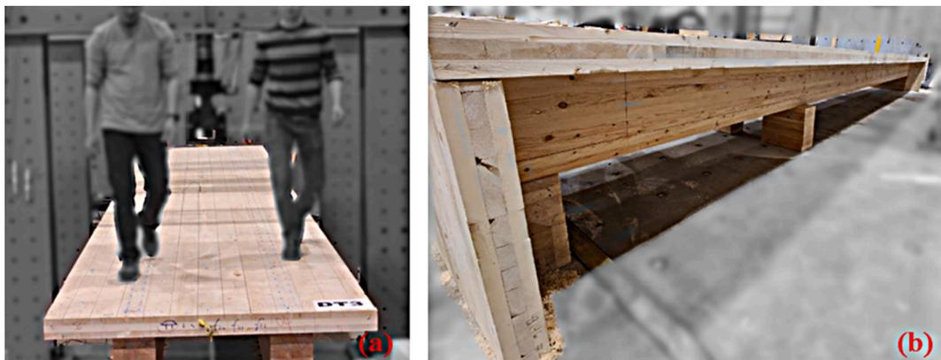
Fig. 8. Walking tests on the T-beam floors (a); specimen with intermediate supports (b).
