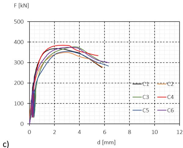
Figure 6. Load-deflection curves: a) Series A, b) series B, c) series C.
