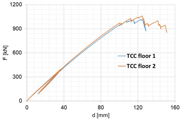
Figure 7. TCC full-scale load-deflection curves
