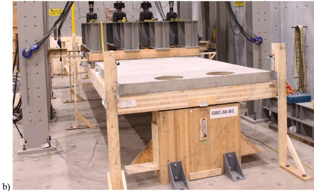
Fig. 5. Schematic (a) and photo (b) of a full-scale bending test setup.
