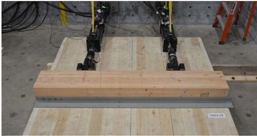
Fig. 6. Setup for ledger tests.
