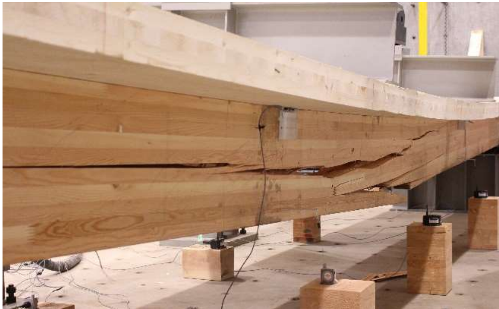
Figure 6: Typical failure in Type A floor specimen
