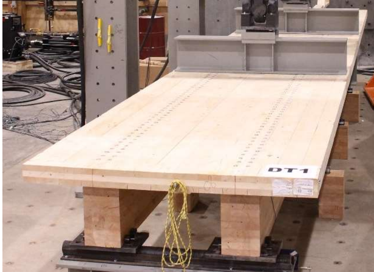
Figure 4: Photo of a 4-point bending test
