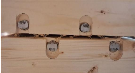
Fig 11: Failure mode series S3
