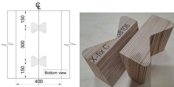
Fig 3: X-Fix connection
