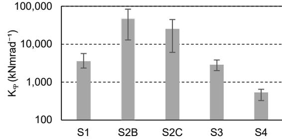
Fig 7: Rotational stiffness of connections
