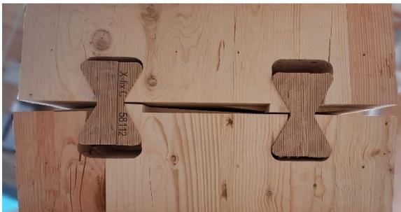
Fig 12: Failure mode series S4
