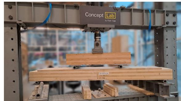
Fig 4: Four-point bending test
