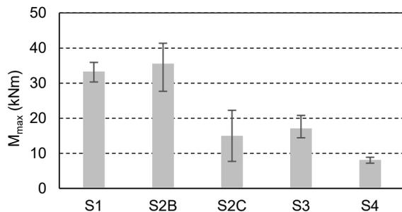
Fig 6: Moment resistance of connections
