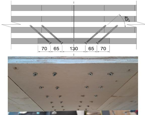
Fig 1: Spline connection with inclined STS
