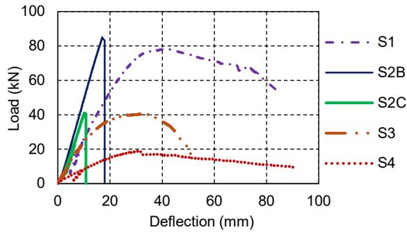
Fig 5: Typical load-deflection curves
