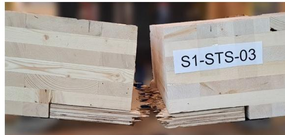
Fig 8: Failure mode series S1
